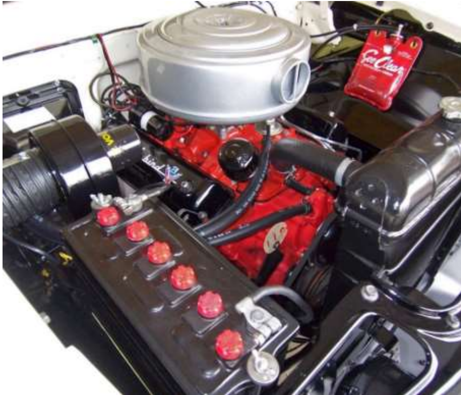
1956 Ford Thunderbird V-8 292-cid 200/202-hp M-code Engine
